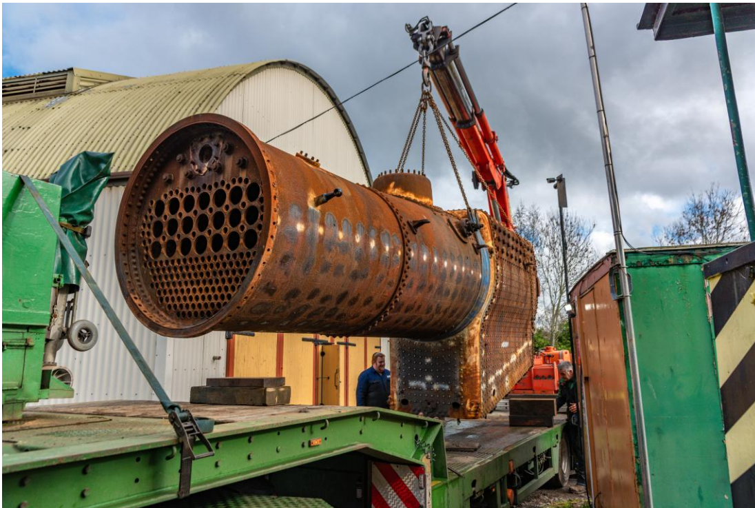
The boiler for BR Standard 4 80064 being transported for restoration
